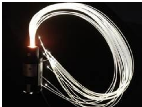
Figure 1. Example of a bundle of LDF's being powered simultaneously from one light source.
